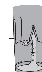
36. With right sides together, pin sleeve into armhole, placing large circle at shoulder seam. Adjust ease. Baste. Stitch, keeping lining free. Stitch again  $\frac{1}{4}''$ (6mm) away in seam allowances. Trim close to second stitching. Press seam allowances flat. Turn seam toward sleeve.
