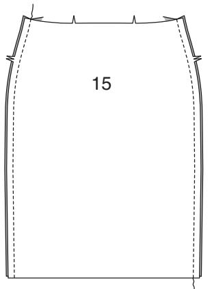
**44.** With right sides together, pin skirt lining to bodice lining, matching centers. Stitch. Press seam toward bodice lining.
