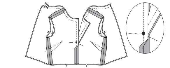
11. Turn lining to inside; press. Baste armhole edge.
