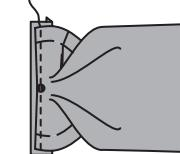
23. Press seam toward continuous lap. Turn pressed edge of continuous lap to inside over seam. **SLIPSTITCH**. Press.
