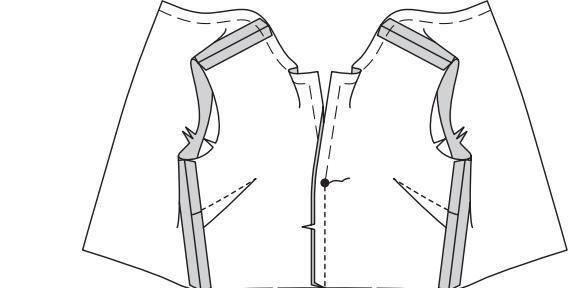
10. With right sides together, pin lining to bodice at neck and front opening edges. Stitch, breaking stitching at large circle, as shown. Trim.
