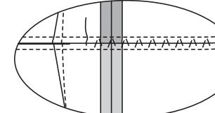
**52.** On outside, pin piping trim to lower edge of dress, having raw edges even, tapering ends to small circle at fold line, as shown. Baste.
