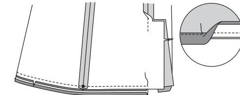
**55.** Turn self facing to inside along foldline, turning up hem facing. Sew hem facing in place. Press. Sew facings to hem facing.
