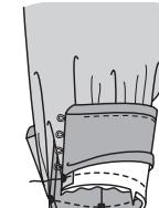
35. **SLIPSTITCH** pressed edge over seam.
