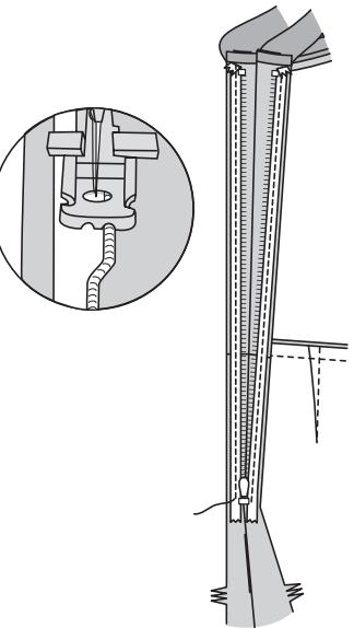
**48.** Close zipper. Slide zipper foot to left. Pin back sections together below zipper. Position and lower needle slightly above and to the left of zipper stitching at large circle. Stitch center back seam between large circle.
