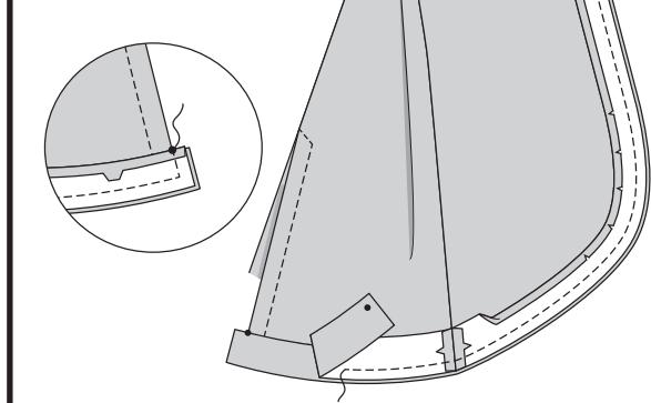
**8.** Turn facing to inside; press. Pin pressed edge of facing 1/8" (3mm) over seam, placing pins on outside. (If you prefer, hand-baste in place and remove pins.) Baste neck edges of band and facing together.
