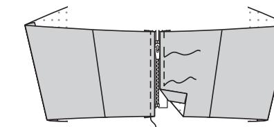
**6.** Fold each SHOULDER STRAP (14) in half, lengthwise, with RIGHT sides together. Stitch, leaving ends open. TRIM seam.
