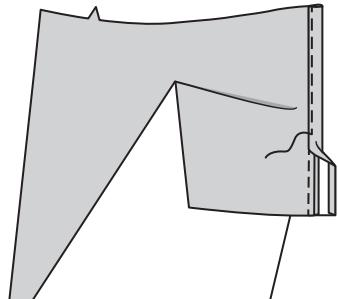
**17.** Turn front edge of lap to INSIDE; baste in place across lower edge. To keep lap in place, stitch diagonally across upper edge of lap as shown.
