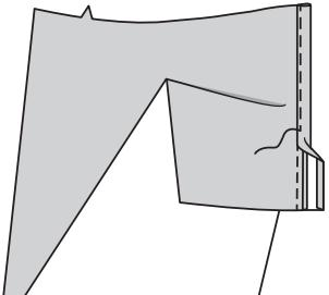
**16.** Pin pressed edge of lap to OUTSIDE slightly over stitching. Stitch close to pressed edge.
