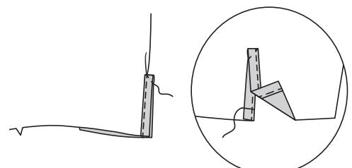
**18.** To make soft pleats, on OUTSIDE, fold along solid lines. Bring folds to broken lines; pin. Baste across raw edge.
