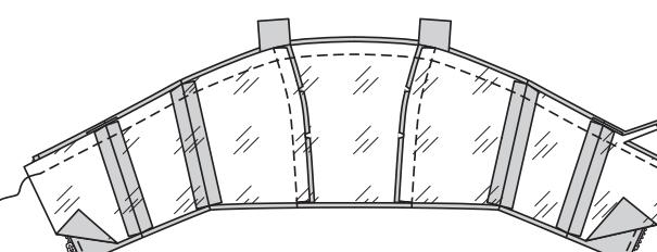
**9.** With RIGHT sides together and raw edges even, pin lower edge of lining to top, matching seams and centers, having lower edges even. Stitch lower edge. TRIM. UNDERSTITCH lower edge of lining as far as possible.
