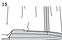
15. Press up  $1-1/4"$  (3.2cm) hem. Press under  $1/4"$  (6mm) on raw edge. Stitch close to inner pressed edge.
