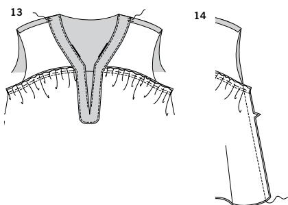
13. **UNDERSTITCH** facing as far as possible. Turn facing to **INSIDE**, turning out ties; press. **TACK** facing to seam allowances to keep it from rolling to **OUTSIDE**.
