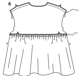
6. Pin back to lower edge of yoke, matching centers and notches. Pull up gathering stitches to fit; baste. Stitch. Press back out, pressing seam toward yoke. Stitch back to front at shoulders.
