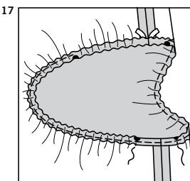
**17.** Smooth casing flat at lower side seam between small and large dots. Stitch across dots to hold elastic in place. Stitch close to lower edge of casing between small and large dots, being careful not to catch elastic.
