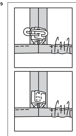
**19.** Lap side front and side back edges of elastic, matching seamlines. Hold with safety pin. Sew lapped edges of elastic with several rows of machine-stitching.
