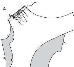
4. With right sides together, pin back to front at shoulders, matching notches and dots. Baste.
