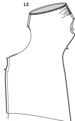
**12.** Stitch front to back at lower left side seam, leaving curved edge free. To keep elastic from getting stuck in the seam allowances as it's inserted, use fusible web or machine-basting to anchor them to dress within the casing area. Be sure to remove basting after casing is finished.
