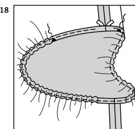
**18.** Smooth casing flat at upper side seam between large dots. Stitch across dots to hold elastic in place. Stitch close to inner edge of casing between large dots, leaving an opening for ends of elastic, as shown, being careful not to catch elastic.
