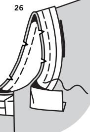
**25.** With right sides together, pin sleeve into right armhole with center small dot at shoulder seam, matching underarm seams, notches and remaining small dots. Adjust ease; baste. Stitch. Stitch again 1/8" (3mm) away in seam allowance. Trim close to second stitching. Press seam allowances toward sleeve.
