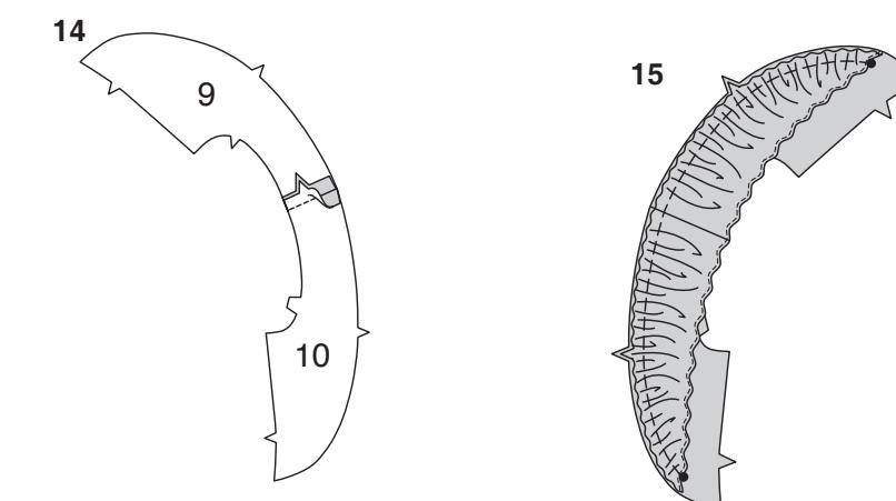
5. Pin RIGHT side of yoke facing to wrong side of back, matching centers; stitch. Press yoke and facing upward.
