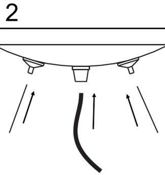
PASS THE CLEAR 3 CORE SUPPLY CABLE AND THE 4 SUPPORT WIRES THROUGH THE CEILING PLATE AS ILLUSTRATED
