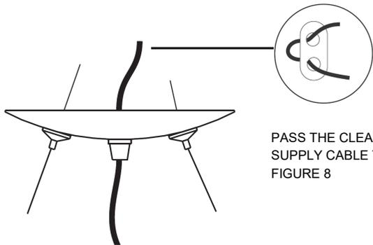
PASS THE CLEAR 3 CORE SUPPLY CABLE THROUGH THE FIGURE 8
