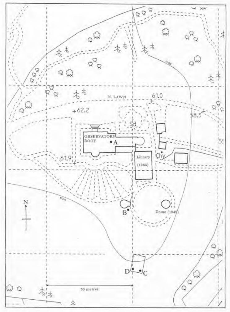
**Figure 1.** Map of the Grounds of Armagh Observatory showing the location of the sunshine recorder since 1880.
