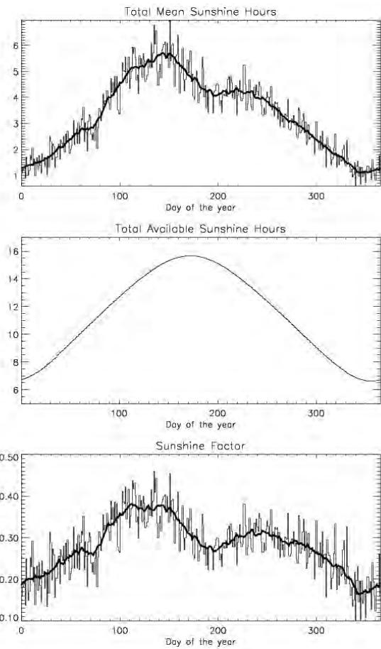
**Figure 3.** The variation of sunshine hours throughout the year at Armagh for the period 1951-1995: (top) Observed daily hours; (middle) Maximum daily sunshine hours; (bottom) The sunshine factor (ratio of observed daily sunshine to the maximum possible).
