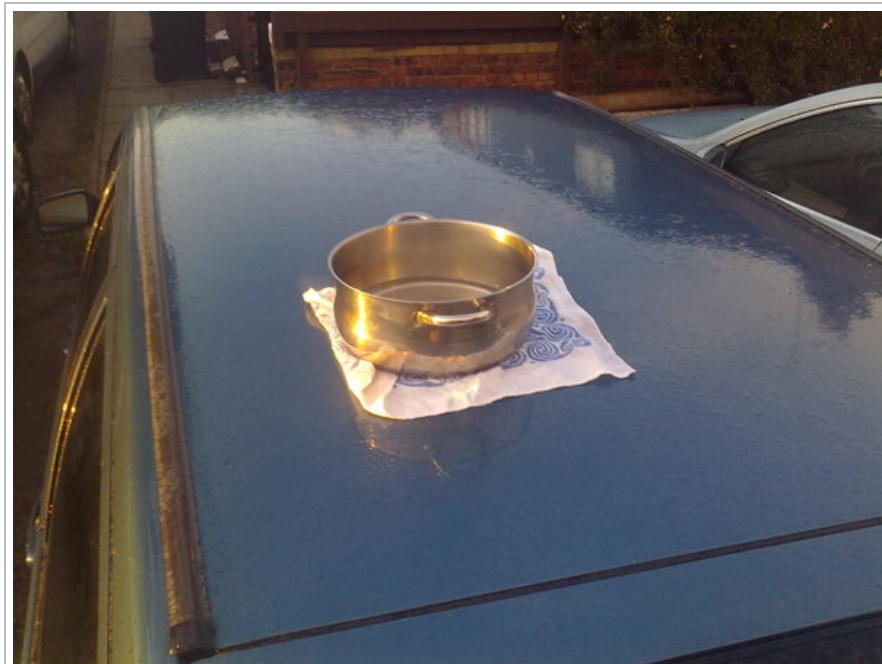
A saucepan can be used to collect wet samples. Place it on a raised surface, away from trees. Here a car roof is used, with a towel to protect the paintwork. Putting water in the saucepan weighs it down and helps it trap ash.
