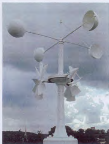
Figure 1. The Robinson Cup Anemometer at Armagh Observatory: the cup anemometer was invented by T.R. Robinson, the third Director.
