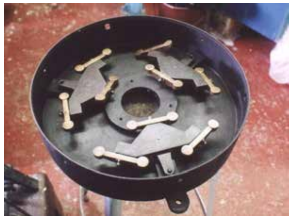
The lever support system for the mirror cell designed by the Dublin telescope manufacturer Thomas Grubb in 1835 for the 15-inch reflector he built, and installed in the 1827 Dome. This compound triangular system is believed to be the first ever to support a mirror this way, and a pre-cursor to the support systems that are now standard for all large optical telescopes.
