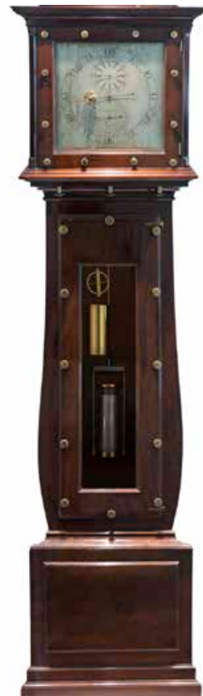
The transit clock built by Thomas Earnshaw for the Observatory on the recommendation of Astronomer Royal Nevil Maskelyne in 1790. Romney Robinson believed it to be the most accurate clock in the world at the time, running to an accuracy of ¼ second per day.
