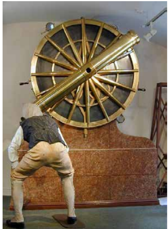
The Jones Mural Circle. Originally used for just measurements of the declinations of stars as they crossed the meridian, using marks engraved on the brass divided circle around it. Later, timing was introduced using a clockwork chronograph to also provide the right ascension. The model is of 3 rd Director Romney Robinson in a typical pose while at work!
