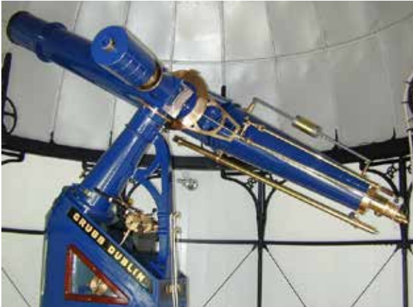
The 10-inch refractor telescope, built in 1885 by Grubb of Dublin, inside the Robinson Memorial Dome. The telescope was used extensively for confirming details of nebulae for Dreyer's New General Catalogue (NGC).
