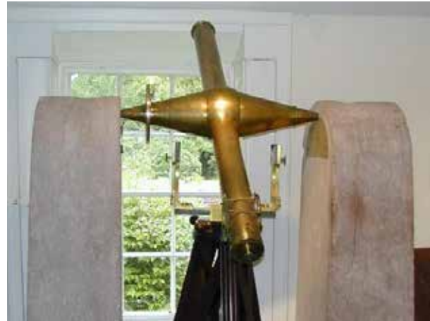
The 3-inch transit instrument built by Thomas Jones in 1827 for timing the transits of stars as they crossed the meridian. Robinson used the instrument extensively for his treatise "Places of 5,345 Stars".
